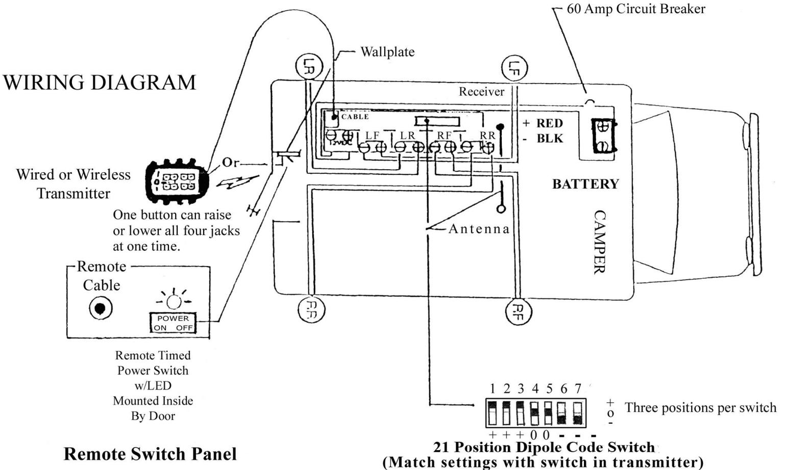
**IN ORDER TO OPERATE THIS ELECTRIC JACK SYSTEM, IT IS NECESSARY TO INSTALL A HEAVY DUTY MARINE/RV BATTERY WITH PROVISION TO KEEP THE BATTERY CHARGED. LOCATE IT IN A SEPARATE SITE, BUT NEAR THE RECEIVER.**
