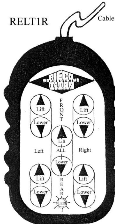
**NOTE: THE BUTTONS ON THE TRANSMITTER FUNCTION AS FOLLOWS: THE "UP" ARROW SIGNIFIES LIFT THE CAMPER, WHILE THE "DOWN" ARROW MEANS LOWER THE CAMPER.**
